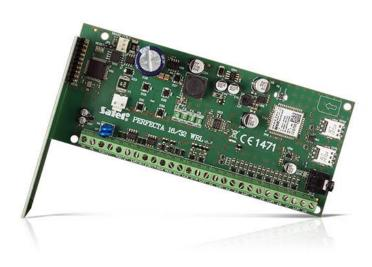
supported to ensure continuity of communication: if any problems occur with the first operator range, the second card is automatically selected.
